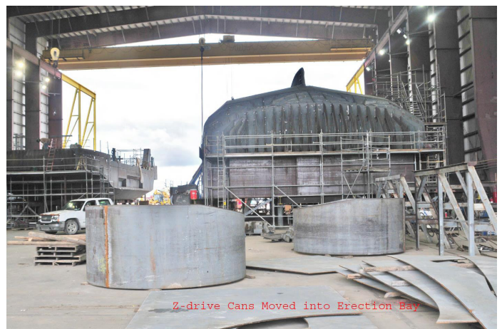
Stern view with Z-Drive cans being prepared for installation.
