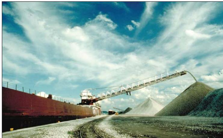
Self unloader laker vessel unloading limestone
